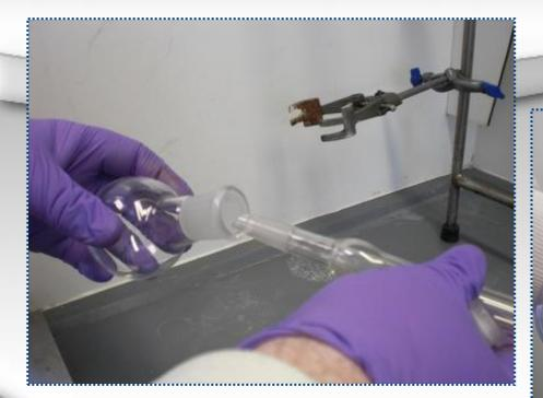
The condenser can not be inserted straight into the round-bottomed flask as the joints are different sizes Always use an appropriate size flask and make sure it is no more than half-full.
