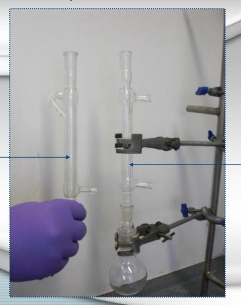
Condenser with screw thread on the glass inlet and outlet pipes
