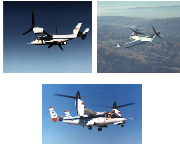
Fig 9 Bell XV-15 Aircraft in Airplane, Conversion and Helicopter modes
