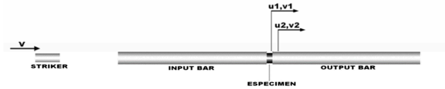
Fig. 2. Schematic of the test fixture for the SHPB test.
