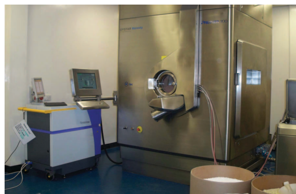
Fig. 2: Photograph of the terahertz sensor unit attached to the production scale film coater.
