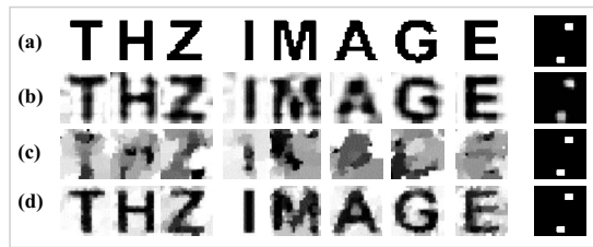
FIG. 3. Simulated results demonstrating the universality of the proposed mask. (a) Original image and reconstructed images using (b) 40 optimized masks, (c) 40 random masks, and (d) 120 random masks.
