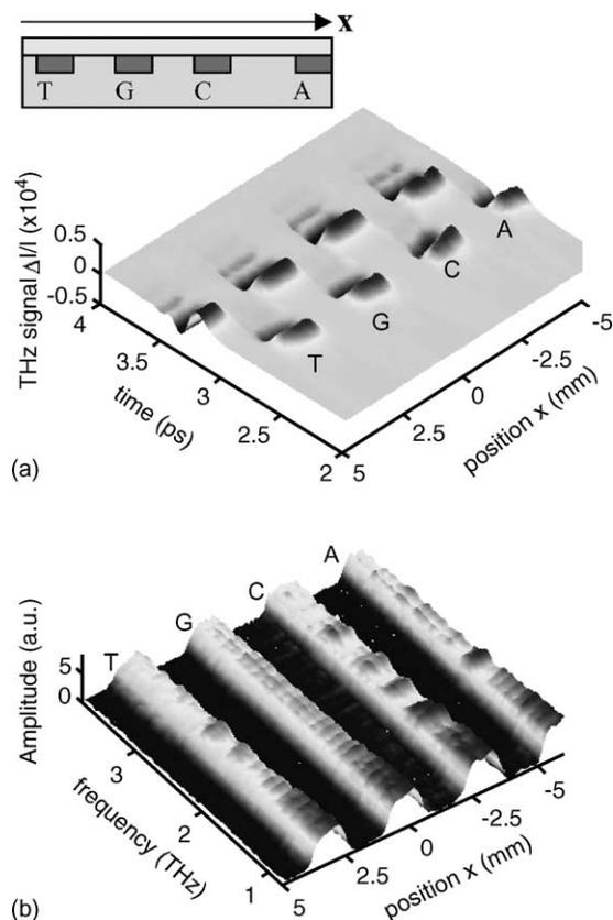
Fig. 4. THz images of nucleosides at room temperature; (a) time-domain and (b) frequency-domain. The inset of (a) shows the schematic structure of the sample for imaging.
