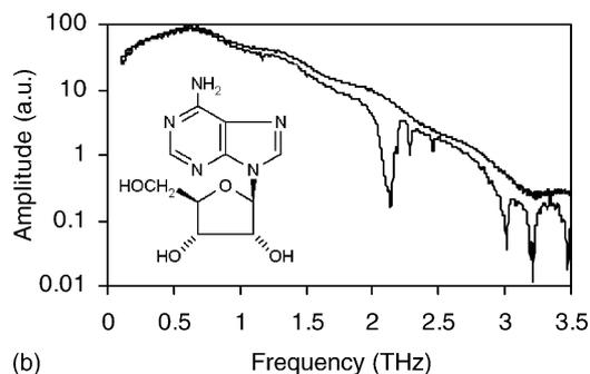
Fig. 2. (a) A typical temporal THz waveform, and (b) its corresponding Fourier-transform amplitude spectrum (upper trace), together with a spectrum measured in the presence of an adenosine sample at 4 K (lower trace). Inset shows the molecular structure of adenosine.
