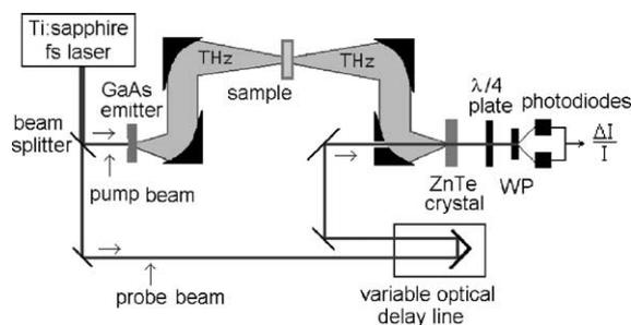
Fig. 1. Schematic representation of the experimental apparatus for coherent generation and detection of THz radiation.
