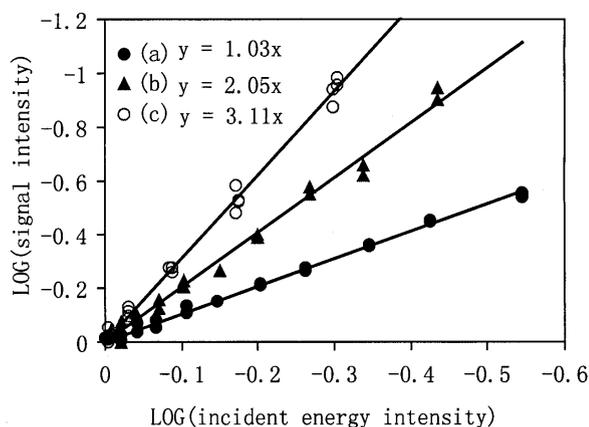
**Figure 2.** The logarithm of the measured signal increase linearly with the logarithm of the pump laser intensity. The slope of the best-fit line is 1.03, 2.05 and 3.11, indicating a linear, quadratic, and cubic dependence on the laser energy for signal from an energy monitor (a), HRS signal of pNA (b) and signal of colloidal gold suspension measured at 400 nm (c), respectively.
