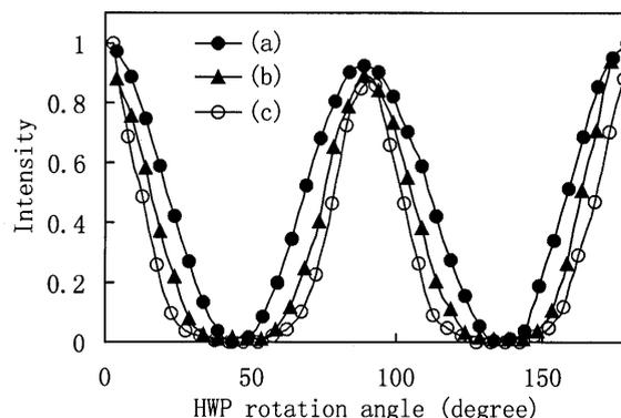
**Figure 1.** The signal intensity change with the HWP rotation angle, (a) signal from an energy monitor, (b) HRS signal measured at 532 nm for *p*NA, (c) 3PF signal measured at 400 nm for colloidal gold suspension.
