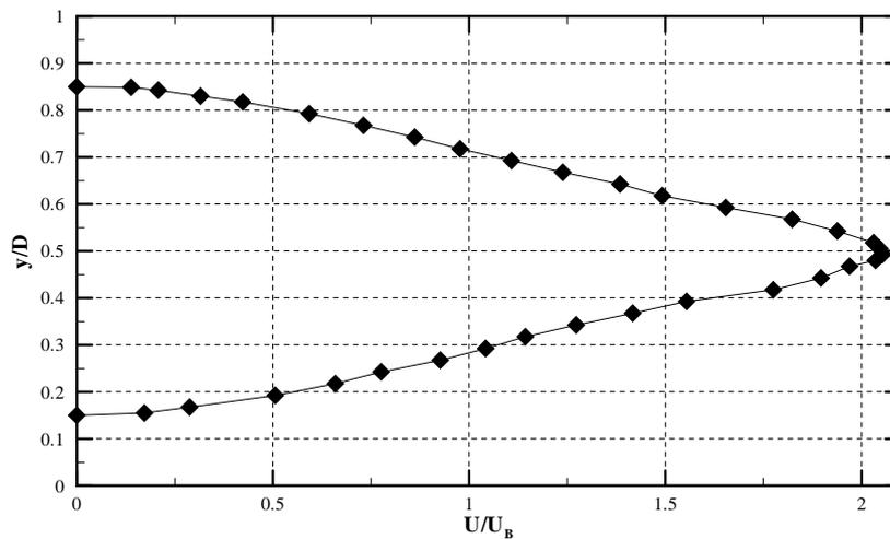
**Figure 5:** Transverse variation of inlet velocity profile in the XY centreplane
