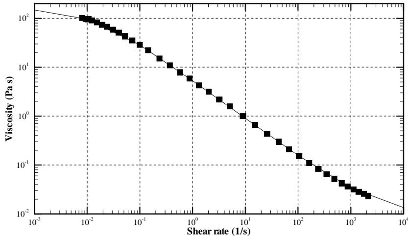
**Figure 2:** Viscosity versus shear rate for 0.4% polyacrylamide (including Carreau-Yasuda fit)
