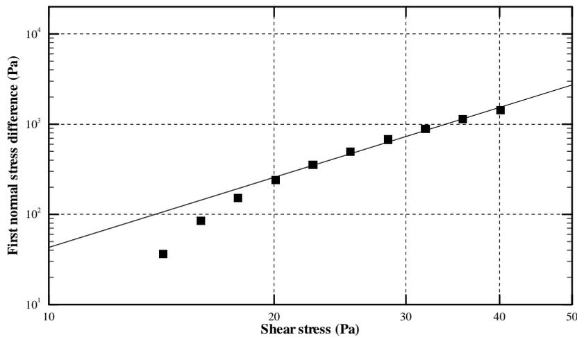
**Figure 3:** First normal stress difference versus shear stress for 0.4% polyacrylamide (including power law fit)
