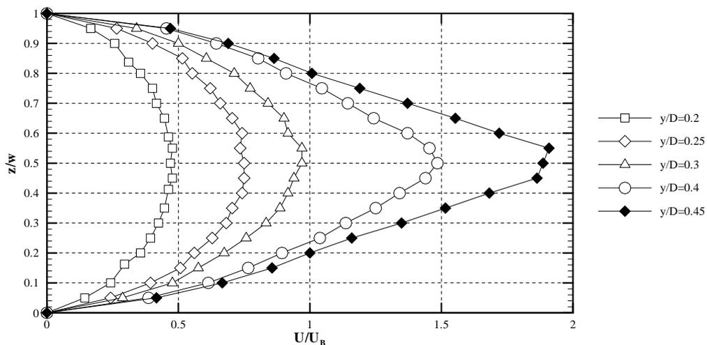
**Figure 6:** Spanwise variation of inlet velocity profile in XZ planes
