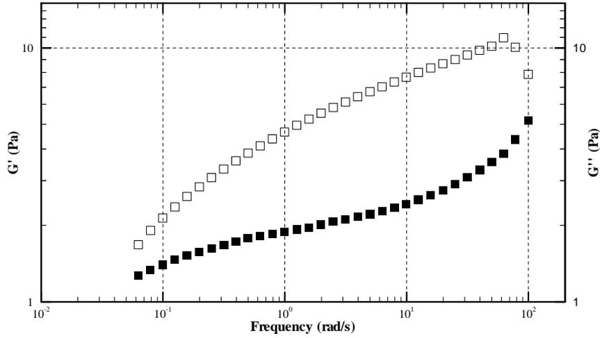
**Figure 4:** Storage ( $G'$  □ ) and loss ( $G''$  ■ ) moduli versus angular frequency for 0.4% polyacrylamide
