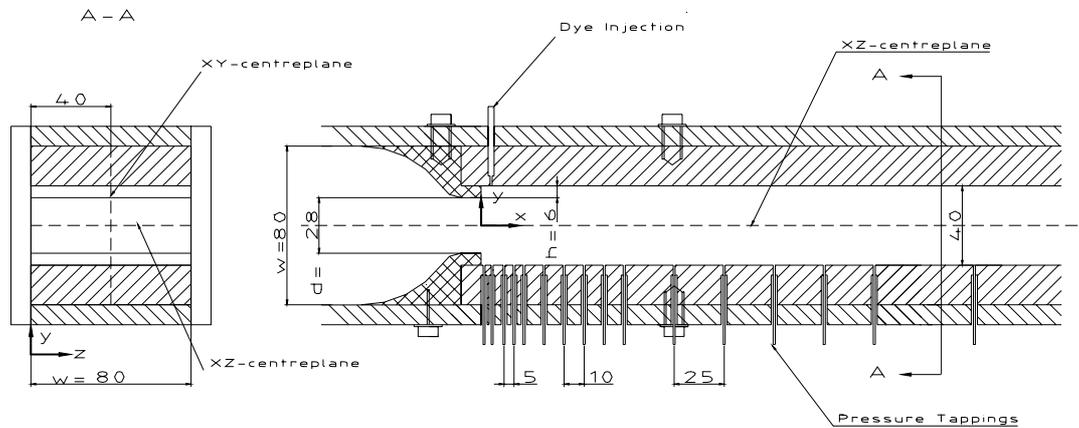
**Figure 1:** Plane sudden expansion geometry, dimensions in mm
