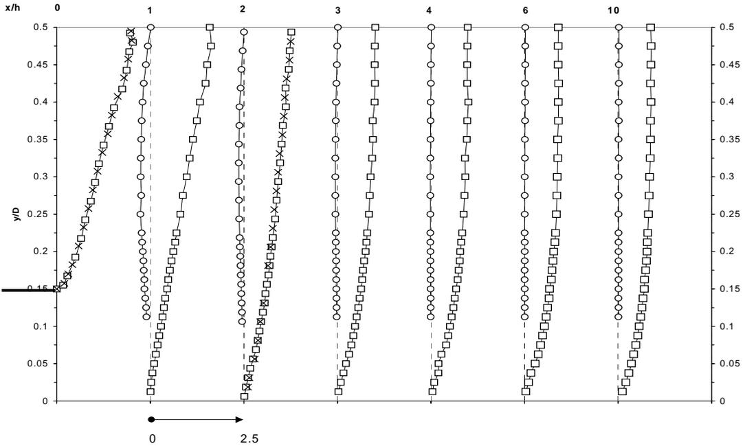
**Figure 7:** Mean axial ( $U/U_B$  □) and transverse ( $V/U_B$  ○) velocity profiles in the XY-centreplane
