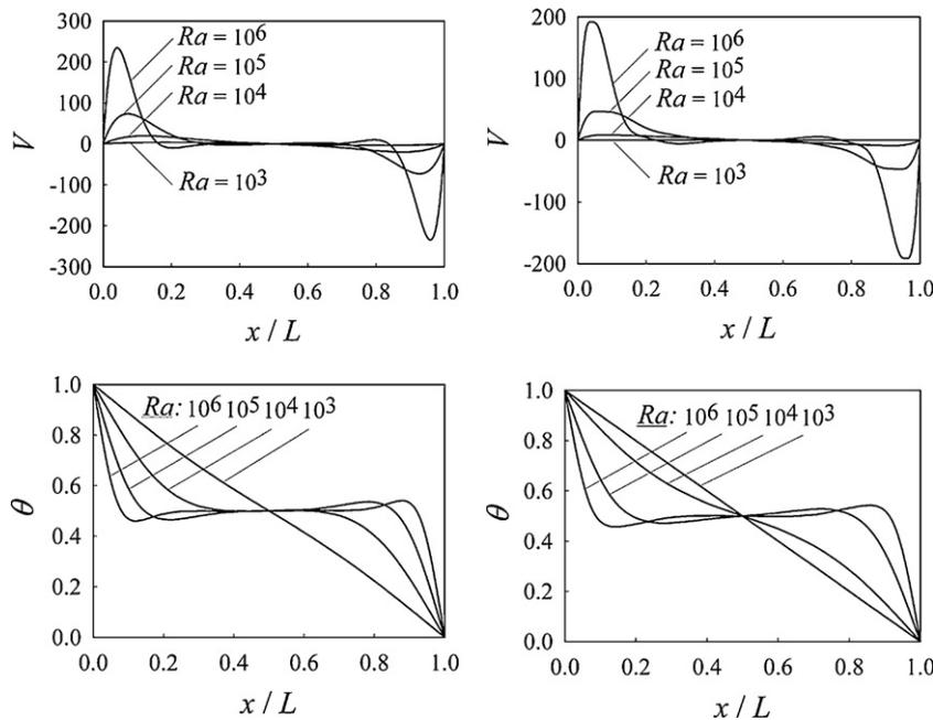
Fig. 3. Variations of non-dimensional temperature  $\theta$  and vertical velocity component  $V$  along the horizontal mid-plane for Newtonian case (left column) and Bingham fluid case (for  $Pr=7$ ).
