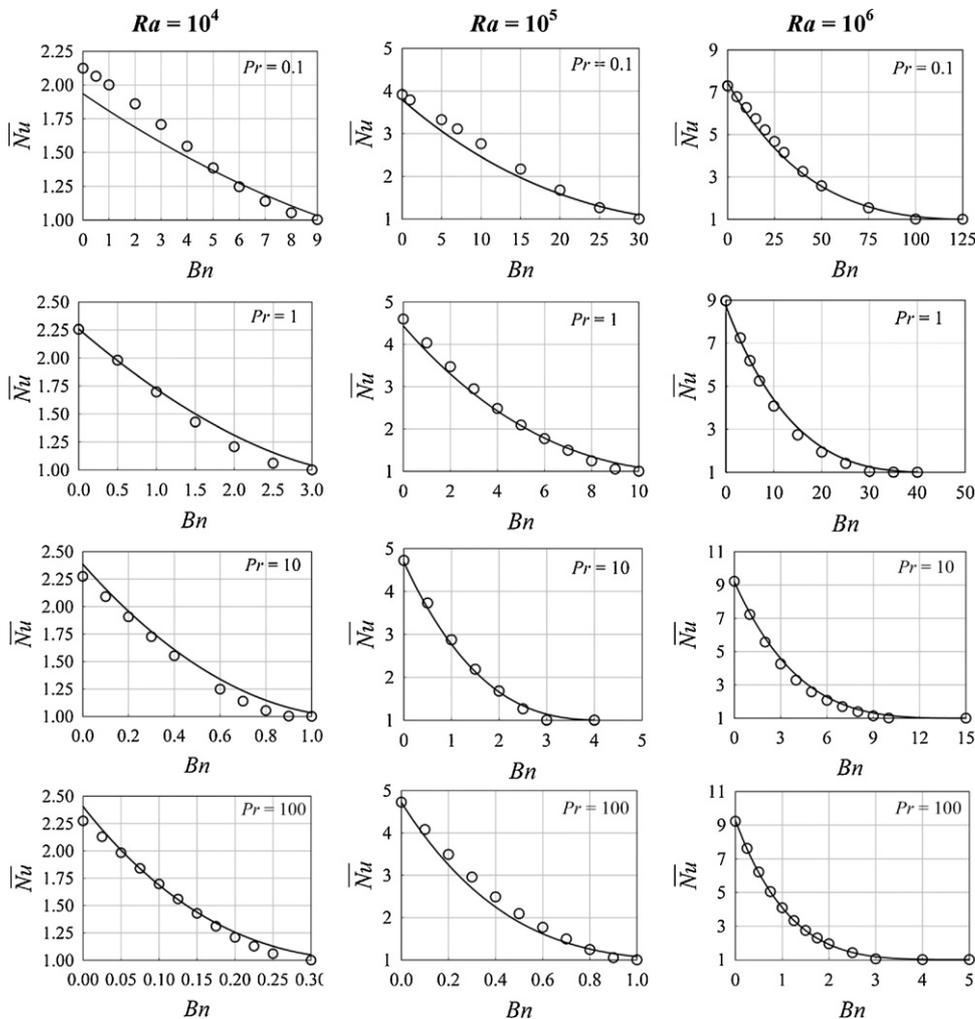
Fig. 12. Comparison of the prediction of the correlation (—) given by Eq. (32) and simulation results (○).
