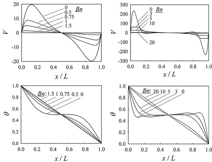
**Fig. 6.** Variations of non-dimensional temperature  $\theta$  and vertical velocity component  $V$  along the horizontal mid-plane for different values of the Bingham number  $Bn$  in the case of  $Ra = 10^4$  (left column) and  $Ra = 10^6$  (right column) ( $Pr = 7$ ).
