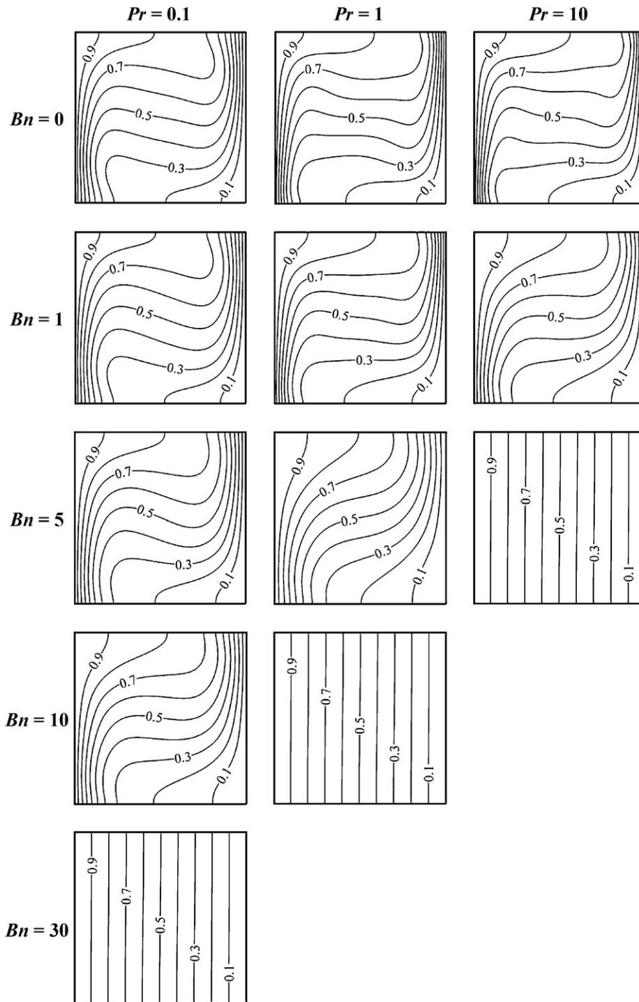
Fig. 10. Contours of non-dimensional temperature  $\theta$  for different values of Prandtl and Bingham numbers at  $Ra = 10^5$ .
