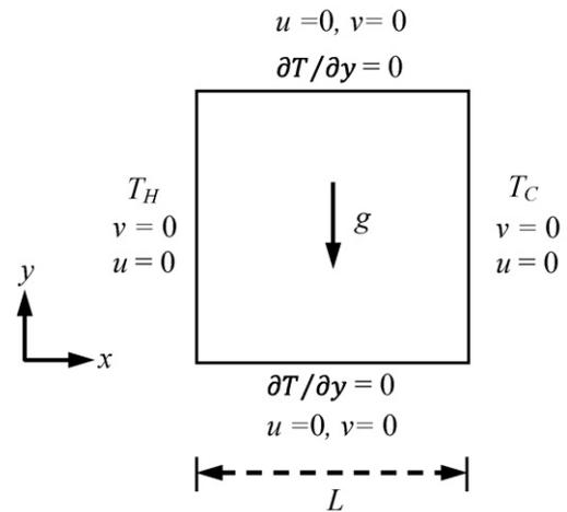
Fig. 1. Schematic diagram of the simulation domain.
