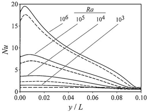
Fig. 2. Variation of  $Nu$  with normalised vertical distance along the hot wall for  $Pr=7$  (–) Newtonian case and (– –) Bingham fluid case (for  $Bn=0.5$ ).
