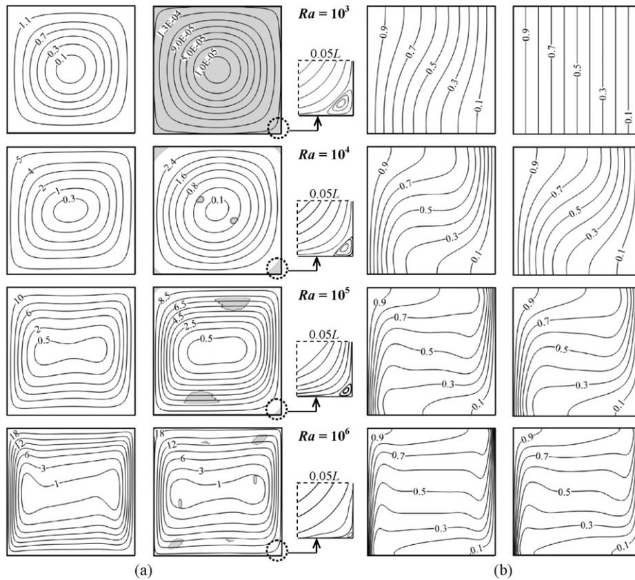
Fig. 4. (a) Contours of non-dimensional stream functions ( $\psi/\alpha$ ) and unyielded zones (gray) including a zoomed inset of qualitative features of corner vortex and (b) contours of non-dimensional temperature  $\theta$  for Newtonian case (left column) and Bingham fluids case (for  $Bn = 0.5$ , right column) at  $Pr = 7$ .
