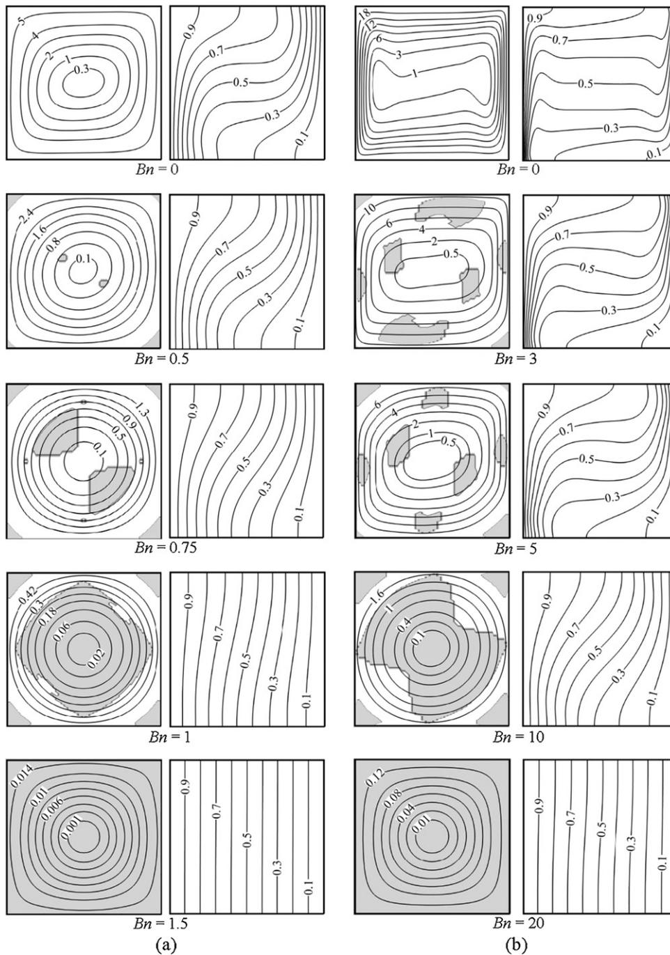
**Fig. 7.** Contours of non-dimensional stream functions ( $\psi/\alpha$ ) (left column) with unyielded zones (gray), and non-dimensional temperature  $\theta$  (right column) for different values of  $Bn$  at  $Pr=7$ , (a)  $Ra=10^4$  and (b)  $Ra=10^6$ .
