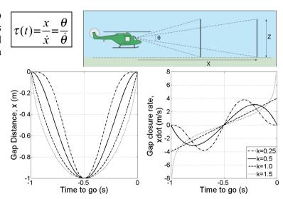
coupled to a tau guide allows the controlled closure of that motion gap with varying accelerationthen-deceleration or varying deceleration motion profiles, as shown in the figure above. In either case, the constant of proportionality (k) determines whether the motion gap closes gently or forcefully.
