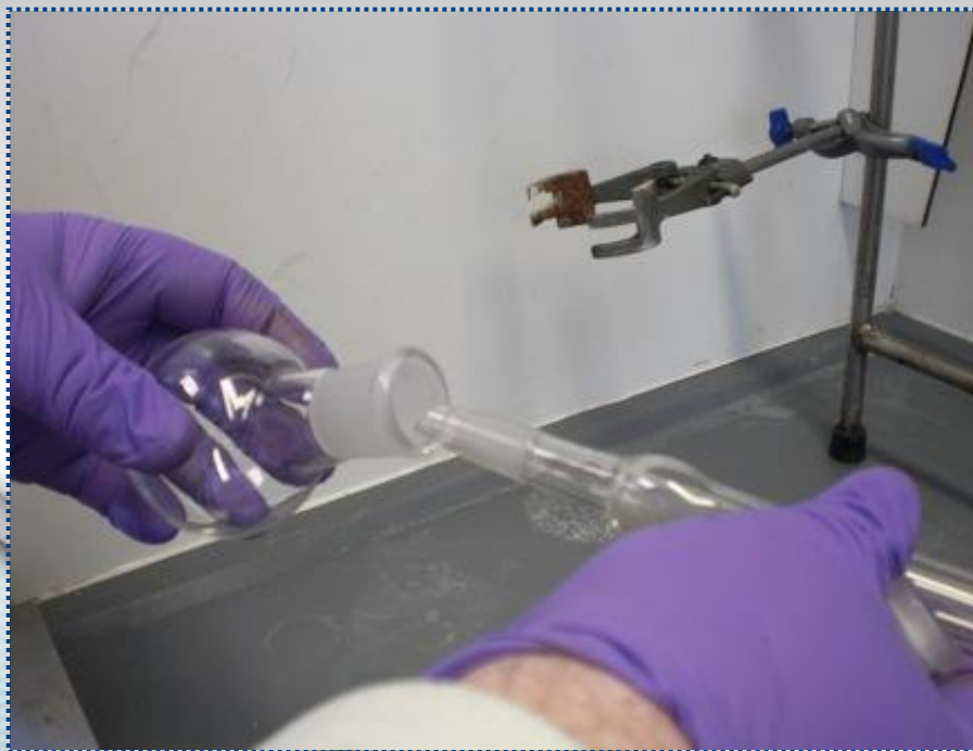
The condenser can not be inserted straight into the round-bottomed flask as the joints are different sizes
