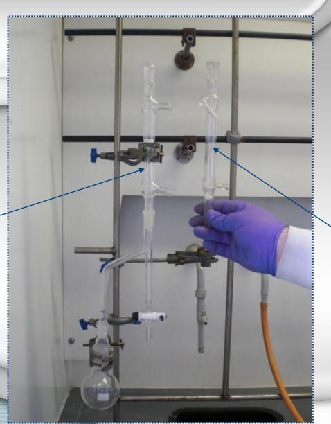
Condenser with glass inlet and outlet pipes with a 'knuckle'
