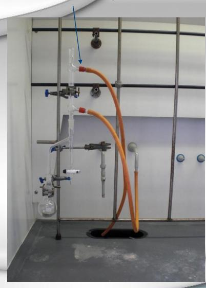
When adding a heat source to the reflux set up, an oil bath may be used instead of the heating blocks. Remember to add either anti-bumping granules or a magnetic stirring bar to the reflux flask. heating blocksheater stirrer
