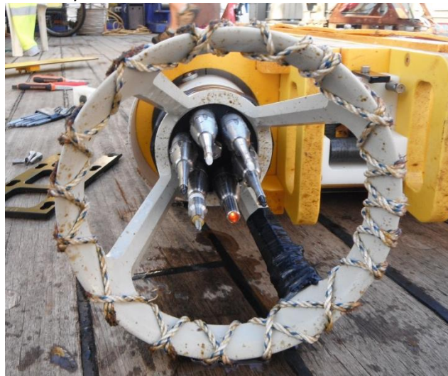
c The recovered MicroRider probes were clean and free of contamination and the MicroRider was still running and recording data after the recovery
