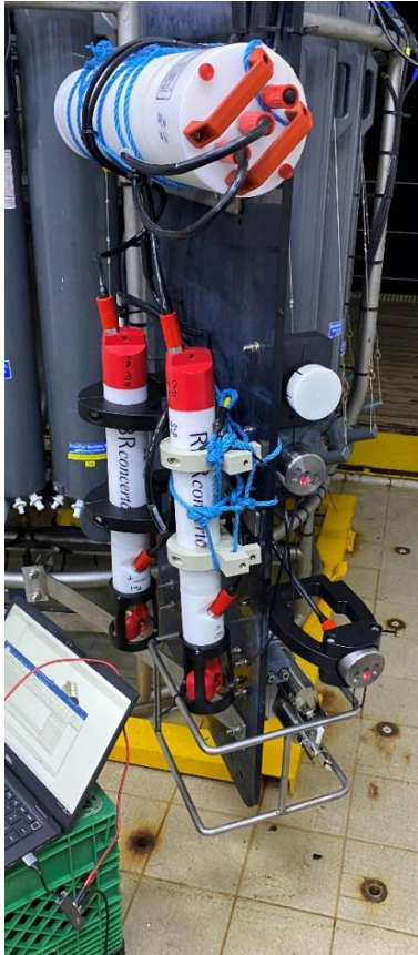
a Both Wirewalker instruments and one RBR Fermata external power battery pack were strapped to the ship's CTD carousel
