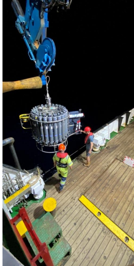
b Deployment of the ship's CTD to 500m with the Wirewalker sensors and battery pack attached on the CTD conductivity cell vane on the right hand side of the carousel
