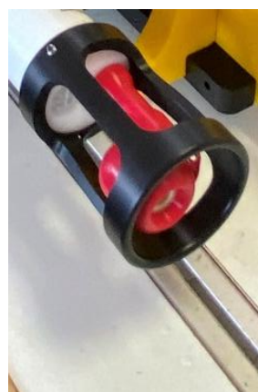
d no obvious fouling of the CTD and PAR sensors shortly after the recovery
