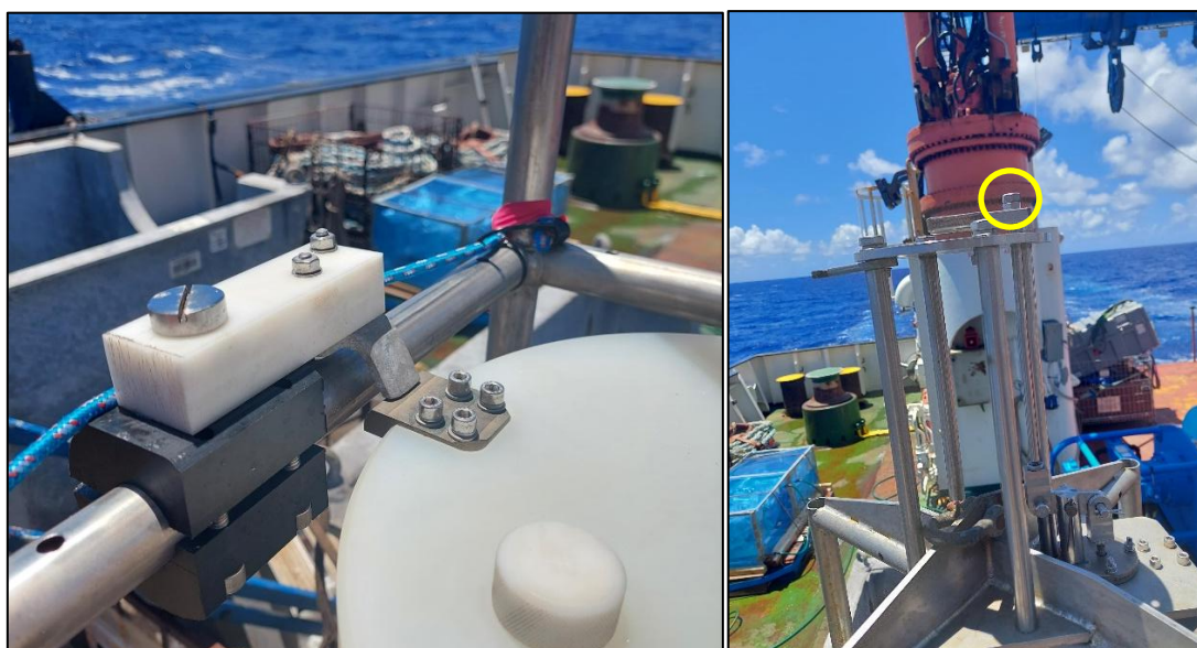
Image 1 (left): a new latch for the lid of Umi to ensure it stays closed once fired.
