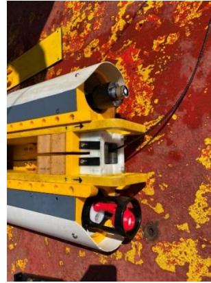
d no obvious fouling of the CTD and PAR sensors shortly after the recovery
