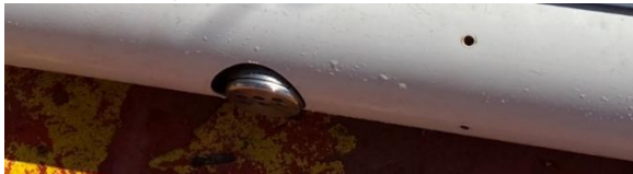
e no obvious fouling of the Trident (Chlorophyll-a, backscatter and fDOM) sensors
