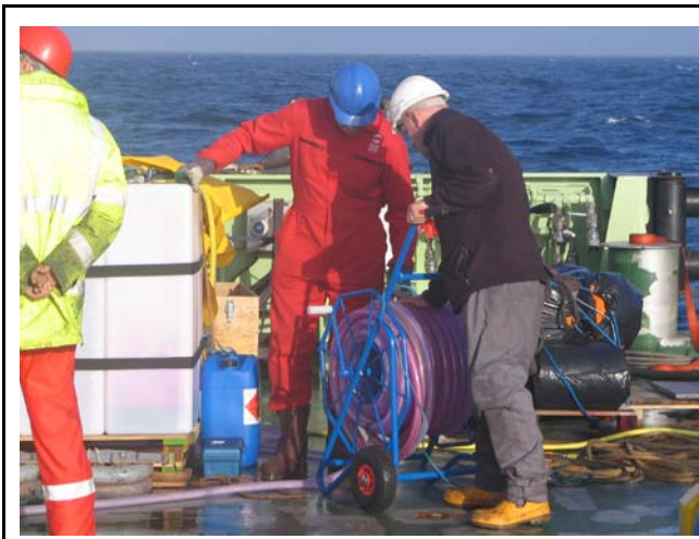
Figure 1: Dye release No. R1. dye mixing and storage tanks next to coiled deployment hose on the aft deck.
