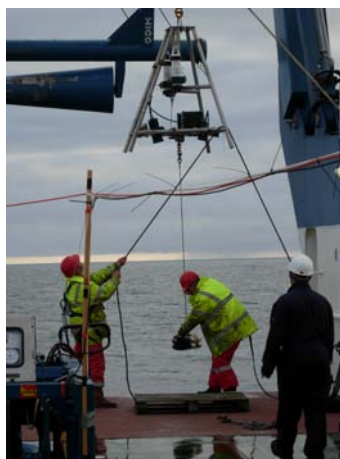
Fig 1 (left). Baited camera frame fitted with camera, flash, battery and acoustic releases.
