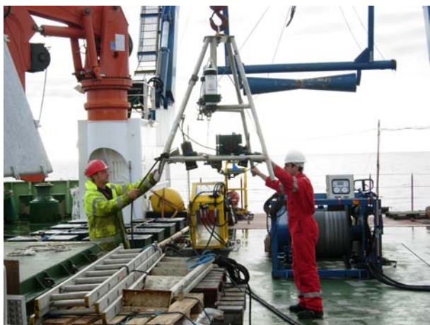
Fig 1 (left). Baited camera frame fitted with camera, flash, battery and acoustic releases.
