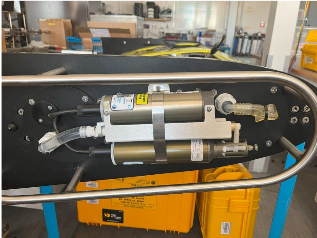
Sea-Bird SBE 3p & 4c Sensor Mounting Location with Forward-facing Exhaust
