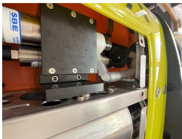
Sea-Bird SBE 43 DO sensor & SBE 5T Pump Internal Mounting Location
