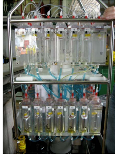
Lugols leaked from bags in RAS-100
