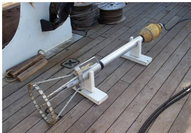
Figure 5.1. The FLY profiler ready for deployment.
