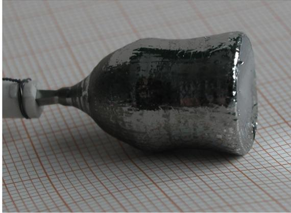
Figure 1.1: A single crystal sample of  $\text{Ga}_3\text{Ni}_2$  grown via the Czochralski method. Note the rotational symmetry of the sample, generated by rotation of the seed at a constant rate during withdrawal from the crucible.
