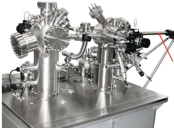
Figure 2.1: An example UHV chamber. Linelock indicated by red arrow
