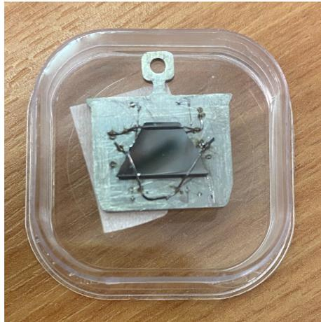
Figure 2.3: A (010) sample of  $\text{Ga}_3\text{Ni}_2$  (shiny material) spot welded to a mounting plate (silver, scratched material), which allows it to be moved without being directly touched.
