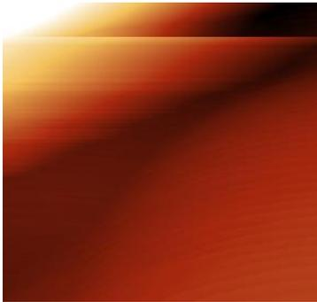
Figure 26: Example of tip not being able to reach into the depths of the surface – a streaking effect is produced as the tip tries to find electron orbits to image.
