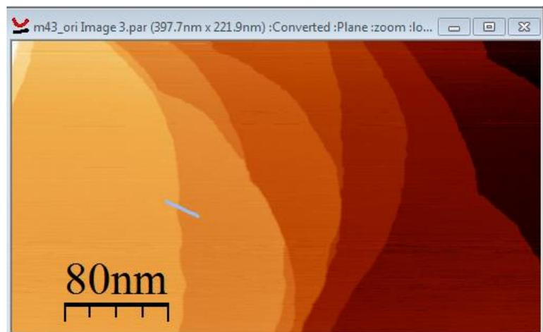
Figure 22: Plane filtered STM image of the 1/1 Ag-In-Yb (100) approximant surface
