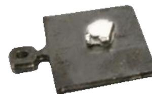
Figure 39: Photograph of 1/1 Ag-In-Yb approximant sample on sample plate: the flat shiny side facing up is the (100) plane.
