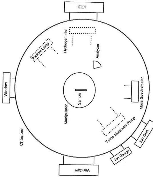
Figure 2.2.1. Experimental UHV Chamber.
