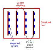
In practice, shielding cannot be complete, because of the need to allow gaps for cooling, and to provide routes for electrical power and signals.
