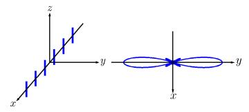
The small "secondary" maxima can be reduced by decreasing the current in the antennae away from the centre; but the principal maxima become wider. The final design is a compromise between the two effects.
