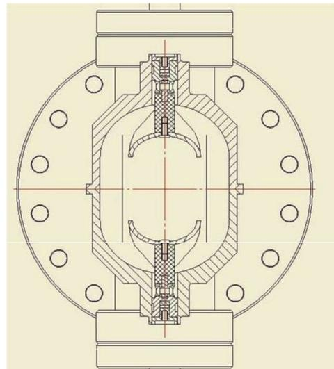
Stripline electrodes developed for fast kicker in DAΦNE.
