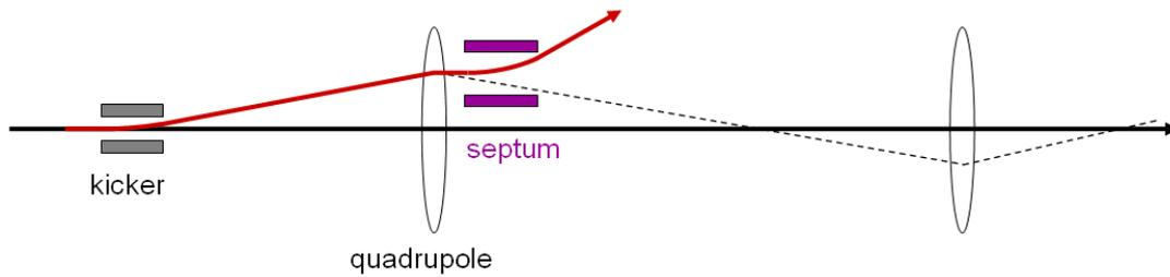
Assuming a distance from the kicker to the septum of 50 m, and a required beam offset from the reference trajectory of 30 mm at the septum, the necessary kick is:
