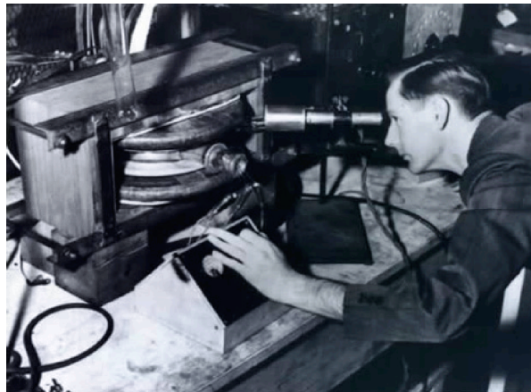
Donald Kirst with the world's first induction accelerator, at the University of Illinois, 1940.
