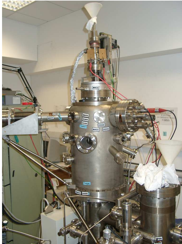
Figure 3.22: The UHV chamber. The optical table has been removed.
