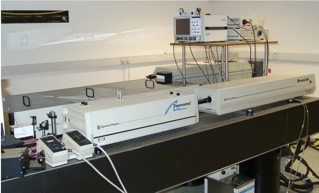
Figure 3.2: Photograph of the laser system, showing clockwise from bottom right: the argon ion oscillator pump laser, the Tsunami femtosecond oscillator, the TSA amplifier and the Nd:YAG amplifier pump laser.
