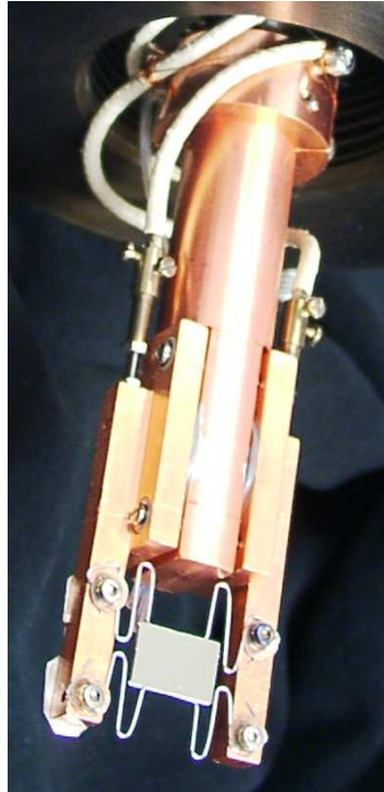
Figure 3.26: Photograph of sample mount and Ru{10 \bar{1} 0} crystal.
