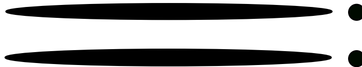
Figure 3.11: Correct light pattern on the compressor grating.
