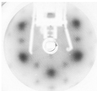
Figure 2.11: (2\times 2) overlayer LEED pattern from saturation O_2 coverage on Ir\{111\} . The background has been reduced to highlight the overlayer spots.
