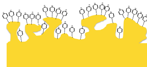
Figure 3.8: A rough gold surface might lead to pyS binding to gold with both the thiol and the nitrogen lone pair.
