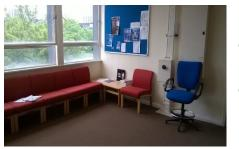
In the main tower, there are parts of the building that have short dead end corridors. These open into small communal spaces (see opposite for example). As a single means of escape, the route should be free from combustibles. Whilst the furniture is likely to offer some resistance in a fire, noticeboards should be class 0 fire resistant and furniture should offer a level of fire resistance.
