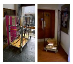
Cages for cardboard were still being stored in the main foyer area. As this is likely to be the main escape route, combustibles in this area should be kept to a minimum. Alternative storage areas for cages containing cardboard should be found. Another cage with cardboard in was found in the stairwell outside the prospectus store area. Those working in this area must be told that cages are not allowed to be stored on the stairwells.
