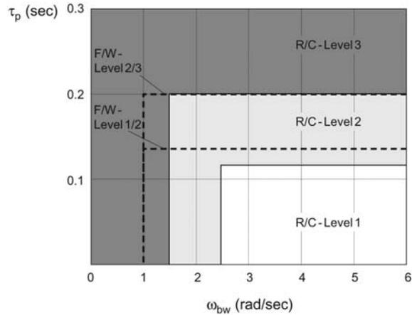
**Figure 8: Comparison of the R/C and F/W roll axis bandwidth criterion**
