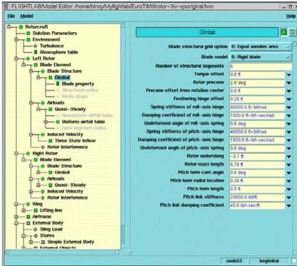
**Figure 11: FLME expanded tree view and data input for the FXV-15 aircraft**
