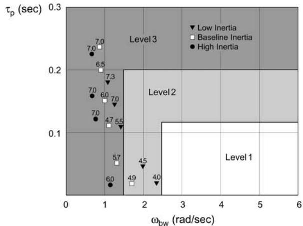
**Figure 21: Comparison of FXV-15 with ADS-33E**
