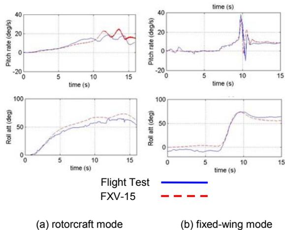
Figure 16: Comparison of the FXV-15 with flight test data [22]
