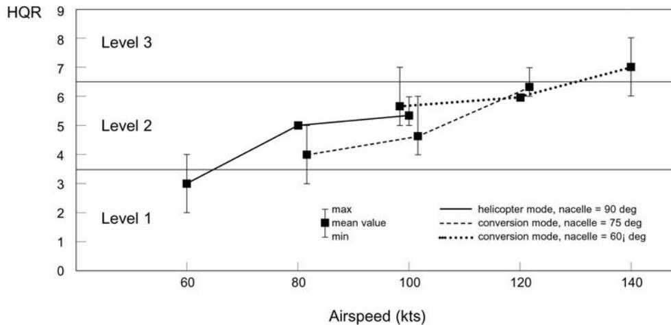
**Figure 19: HQRs for the roll-step maneuver**
