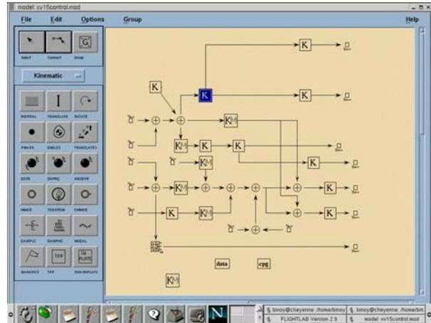
Figure 10: GSCOPE representation of the FXV-15 collective lever and lateral stick channel
