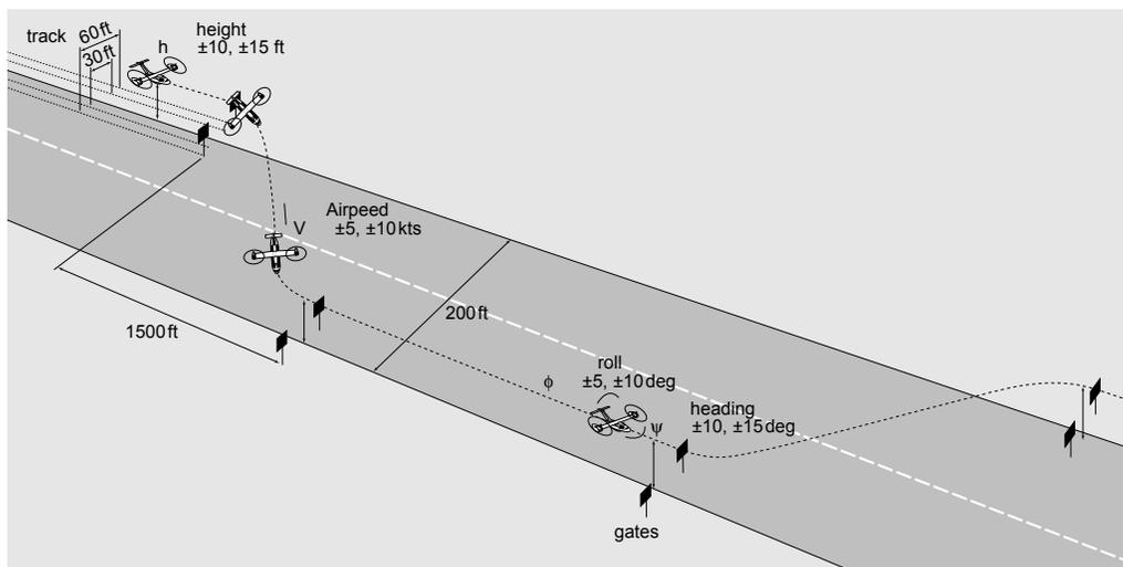
**Figure 6: Layout of the roll-step Handling Qualities test maneuver**
