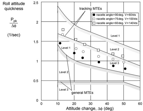
**Figure 18: Roll attitude quickness for the FXV-15 in rotorcraft and conversion modes**
