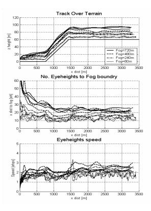
Fig 7 Flight trajectories and eye-height parameters for terrain hugging manoeuvres
