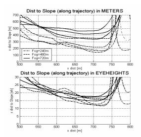
Fig 8 Distance to the slope surface (in meters and eye-heights)
