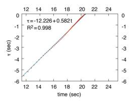
Fig 2 Regression fit of  $\tau$  vs time for helicopter in quick-stop manoeuvre (Ref 10)
