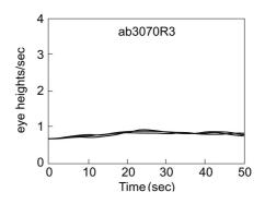
Fig 5 Aircraft velocity in eye-heights/sec over flat terrain (initial conditions, 30kts, 70 feet agl)
