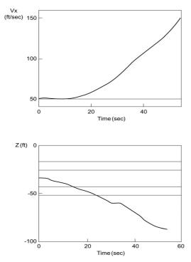
Fig 6 Aircraft velocity and height over flat terrain (initial conditions, 30kts, 70 feet agl)
