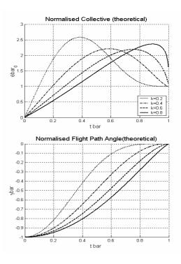
Fig 15 Normalised collective pitch and flight path response following a constant acceleration  $\tau$  guide
