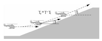
Fig 10 Flight path angle
