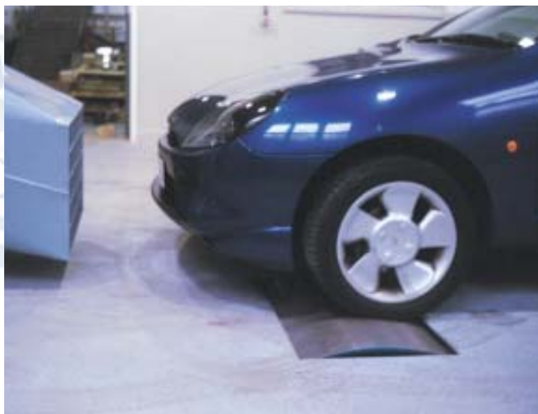
The Liverpool Rolling-road Dynamometer Measuring the Torque and Speed at the Wheel
