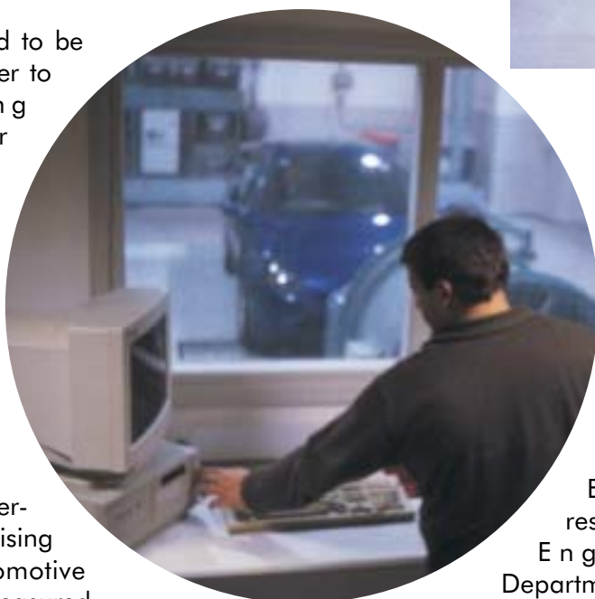
Measuring vehicle performance on the Liverpool Rolling-road Dynamometer
