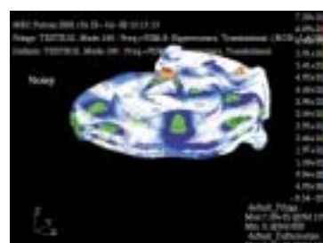
Predicted Noisy Mode at 9206Hz
