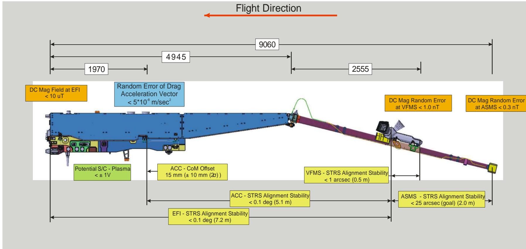
**500kg incl. 99kg fuel; ~1.0 m<sup>2</sup> cross section 4 years lifetime**
